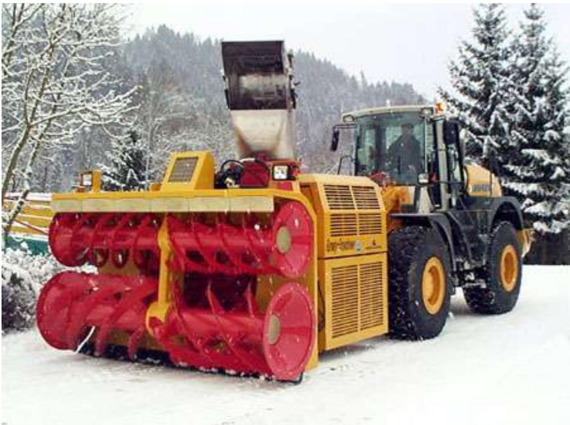
DOBLE FRESADORA FRONTAL CON MOTOR INDEPENDIENTE
