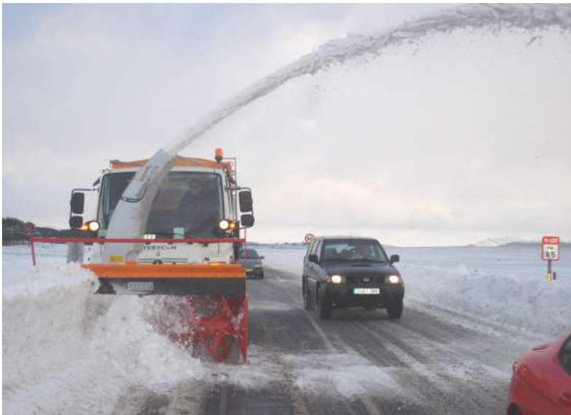
FRESADORA FRONTAL ENSANCHANDO CALZADA
